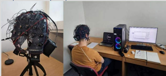
Fig. 1: The EEG device from g.tec used for measurements
