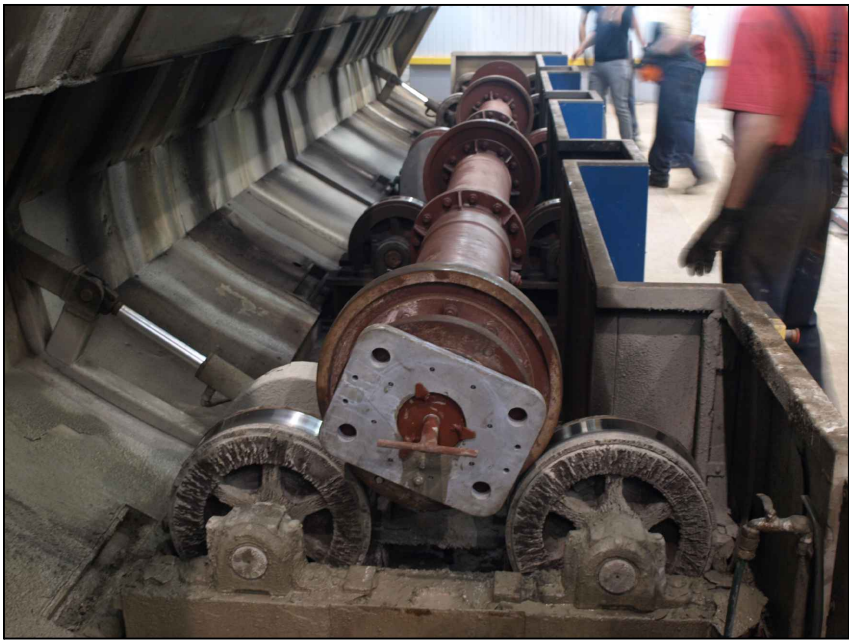
Fig.7. A concrete mould filled with a concrete mixture in a roller centrifuge
