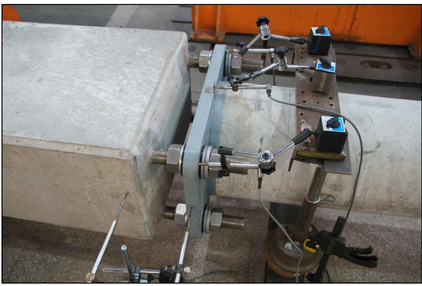
Fig.11. Fastening of the ETG-3 pole to the pile foundation with measuring instrumentation
