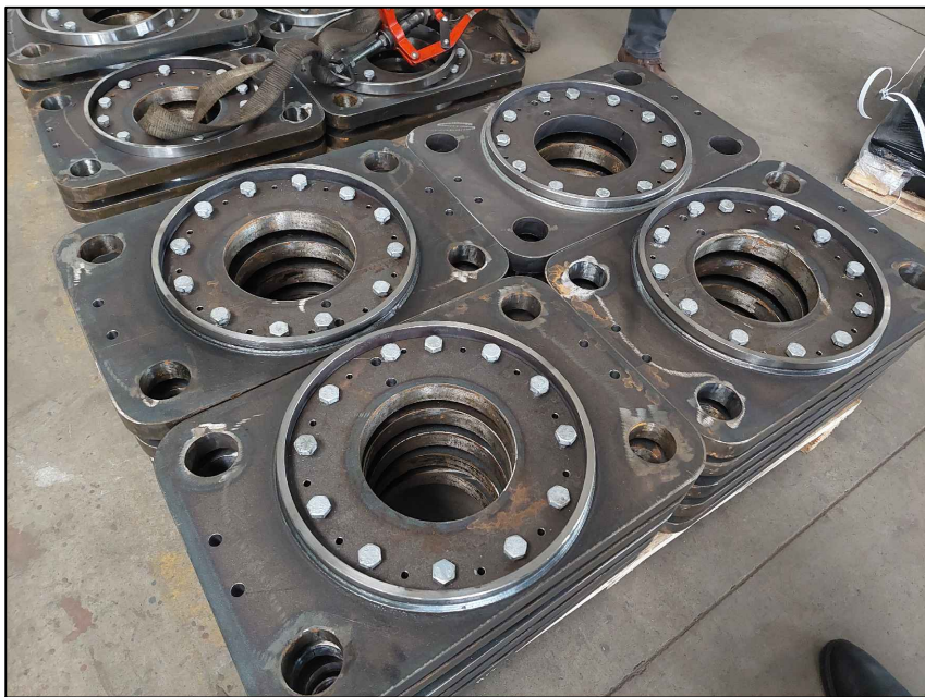
Fig.2. Steel heads of railway traction poles prepared for galvanizing
